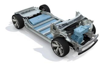
Renault's future all-electric vehicles will be built on the new modular CMF-EV platform designed by Renault-Nissan-Mitsubishi, making each new model easier to manufacture with increased and optimised electric performance.
